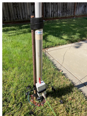
Figure 1. Base of the antenna showing the mast, radial connections, and matchbox.
